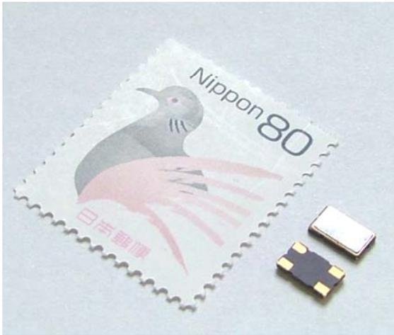
The ACU6035 is a common 6.0 x 3.5mm SMD package with seam welding. This highly reliable, stable, and accurate device is suitable for Digital AV devices, Clock source of IC, mobile telecommunication applications.
